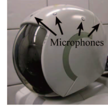
Fig. 5. The microphone layout on ASIMO's head. The eight microphones forms like circle.
