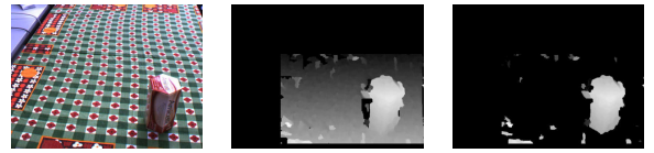
Fig. 5: Results of plane subtraction. Left column : Original color image. Middle column : Disparity image of the color image on its left. Right column : Remaining object in the disparity image after the plane subtraction.
