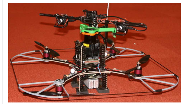
Fig. 1. Our quadrotor helicopter. Sensing and computation components include a Hokuyo Laser Rangefinder with laser-deflecting mirrors for altitude, a pair of stereo cameras, a monocular color camera, an IMU, and an Intel Atom based flight computer.
