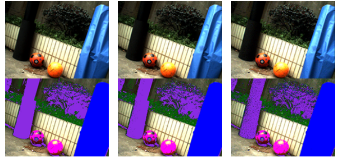
Fig. 4. The typical images along ridge curve and the processing results in outdoor experiment. (top) are the typical images. (bottom) are the processing results. The camera parameters are as follows: (left) exposure time: 22ms, gain: 9. (middle) exposure time: 14ms, gain: 14. (right) exposure time: 7ms, gain: 22.
