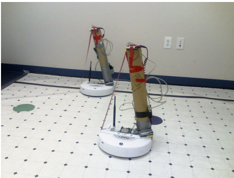
Fig. 7. Two LANdroids robots with added compasses (mounted on tall cardboard pipes to reduce magnetic interference from ground and robot).
