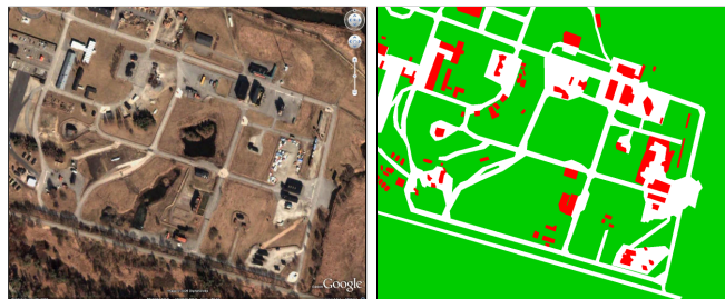
Fig. 1. Map over the operational environment obtained from Google Earth™ (left) and a manually classified reference map with grass, asphalt and houses as prespecified classes (right).
