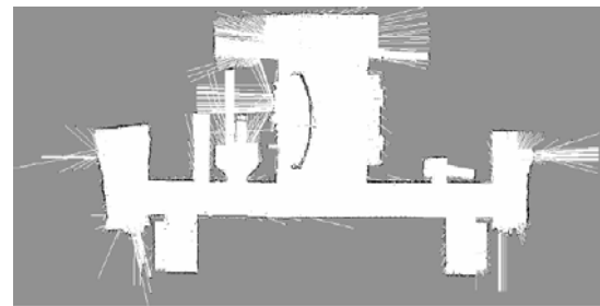
Fig. 4. Result of map building by FastSLAM
