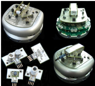
Fig. 4. Khepera III and KheNose with sensing modules
