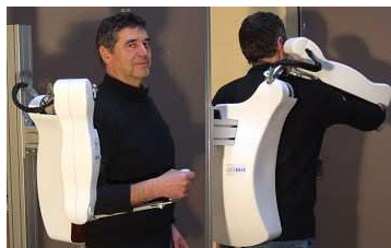
Fig. 5. ABLE 4 axis exoskeleton actuated by screw-and-cable actuators
