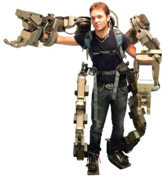
Fig. 1. The fully actuated body extender developed at PERCRO
