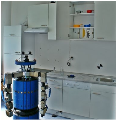
Fig. 6. The B21 robot in the kitchen, with RFID readers visible inside the cabinets.
