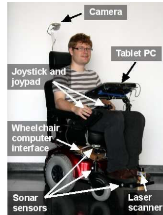
Fig. 1. Global localisation data from the camera is used alongside dynamic sensory data from the laser scanner and sonars to assist the user in performing precise manoeuvres. In this experiment, the user controls the wheelchair using the joystick in their right hand, whilst performing a secondary task on the joypad buttons with their left hand.
