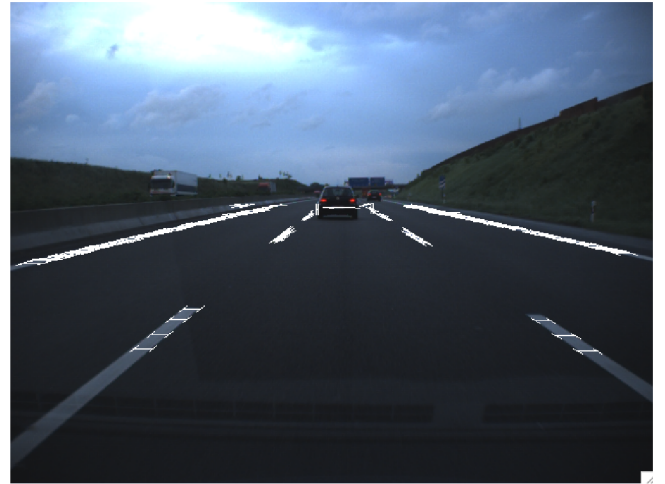
Fig. 7. Extracted marker widths for multiple lanes in the image plane.
