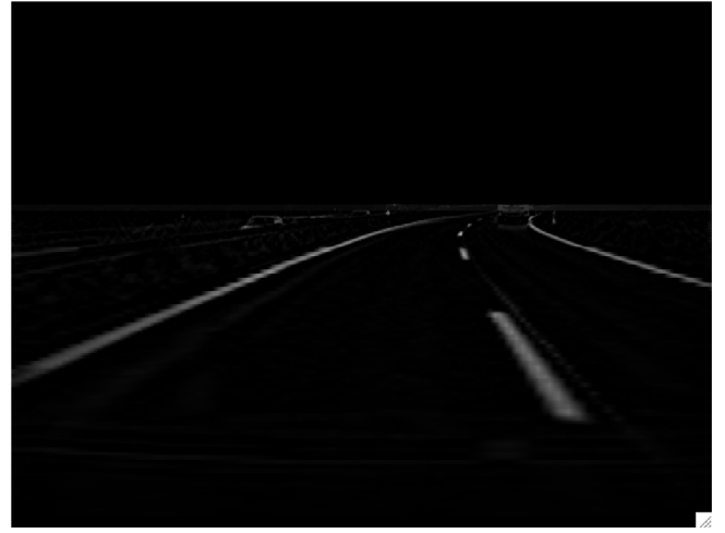
Fig. 2. Result of filtering a grayscale camera image with the marker extraction mask.
