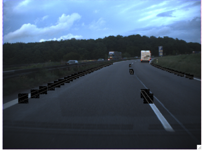
Fig. 3. Edge intensity in ROIs used for marker gradient and marker width estimation.
