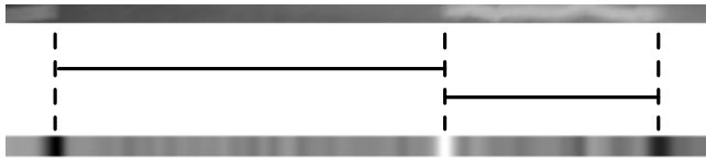
Fig. 8. Top row shows a marker strip image generated from lane marker candidate positions. Bottom row shows the result of applying a Prewitt filter to the vertically averaged image. Lines indicate gap- and marker length.
