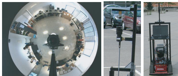
Fig. 8. Example image (left), omnidirectional camera (center) and complete setup (right) used for the experiments.
