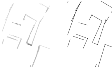
Fig. 4. Segment merging. Clusters of segments (left) are replaced by single representative segments (right). The figure shows a magnified view of the center of Figure 5 b) and c).
