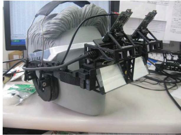
Fig. 4. Stereo HMD for Simple PH System
