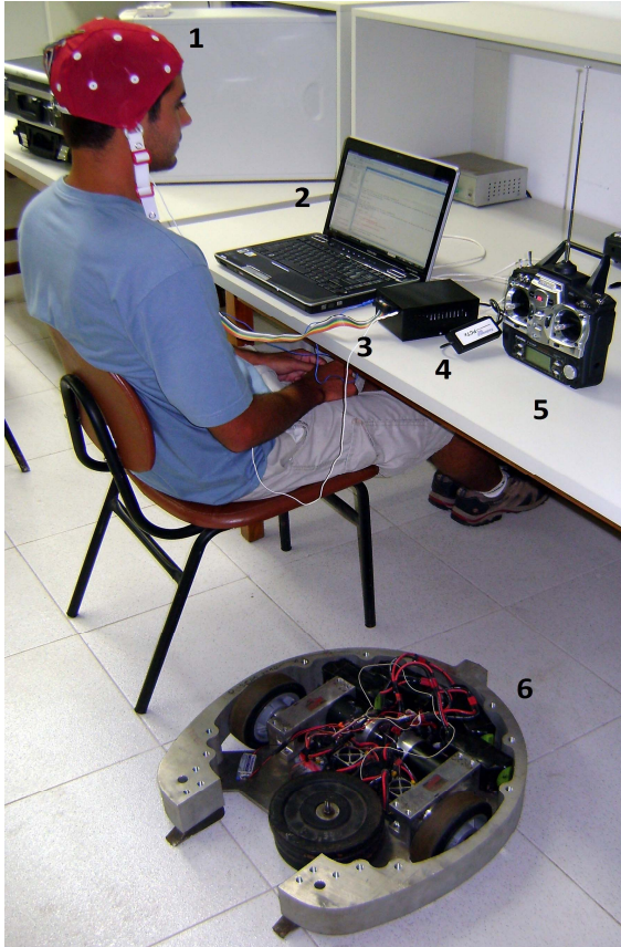
Fig. 8. Experimental system: 1- Electrodes; 2- Computer; 3- EEG System in metal enclosure; 4-PCTx link; 5- RF Transmitter; 6- Mobile Robot.
