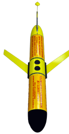
Fig. 1. HeHaPe, one of two USC Slocum gliders.
