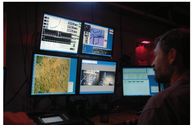
Fig. 6. WHOI research engineer Matthew Heintz remotely pilots Nereus during Dive 10. Vehicle controls and displays include (from lower left) robot manipulator master control, high-resolution imaging camera display, depressor navigation and control panel, vehicle navigation display, vehicle control panel, and utility camera displays.
