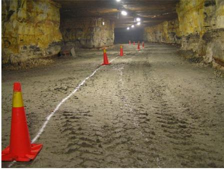
Fig. 5. A tunnel with a painted white line indicating a simulated ditch.
