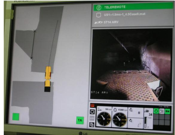
Fig. 6. OPS display with local autonomy functionality active. The yellow shape with a black rectangle on the left represents the machine and the bucket. The dark gray areas are the free areas sensed by the laser scanners. The calculated path is shown by the thin line above the machine, and the detected side tunnel by a black line with x at its ends.
