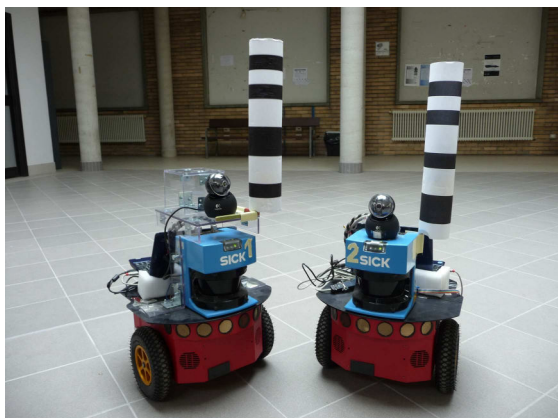
Fig. 4. Robots P3-DX used for real test. A bar code marker is used to distinguish the robots.
