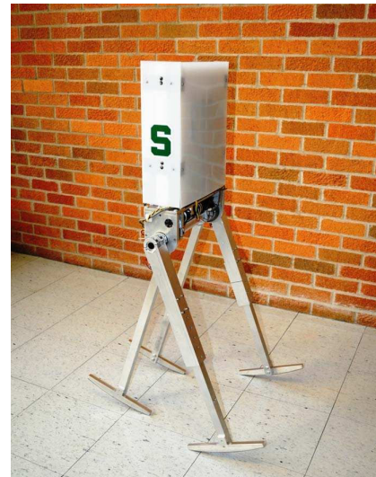
Fig. 3. The synthetic wheel biped developed at Michigan State University
