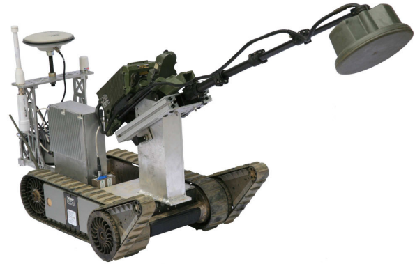
Fig. 1. A photograph of the modified PackBot Fido from iRobot used in tipover validation tests.
