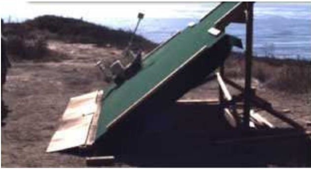
Fig. 2. A video frame of the robot driving up at 40^\circ ramp during a tipover test.
