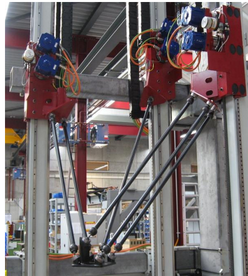
Fig. 1. The full-scale F1 Parallel Kinematic Manipulator at Güdel AG, Langenthal, with dual motor control on each cart for overall increased accuracy and stiffness.
