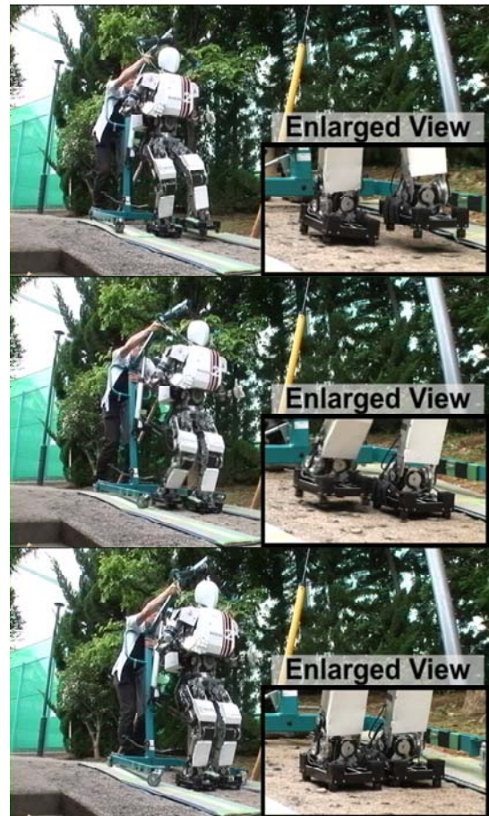
Fig. 14. Walking experiment outdoors. The maximum angle of inclination is 7.0 degrees and the maximum height of unevenness is 15 mm. The walking cycle is 1.0 s/step with a step length of 200 mm/step.
