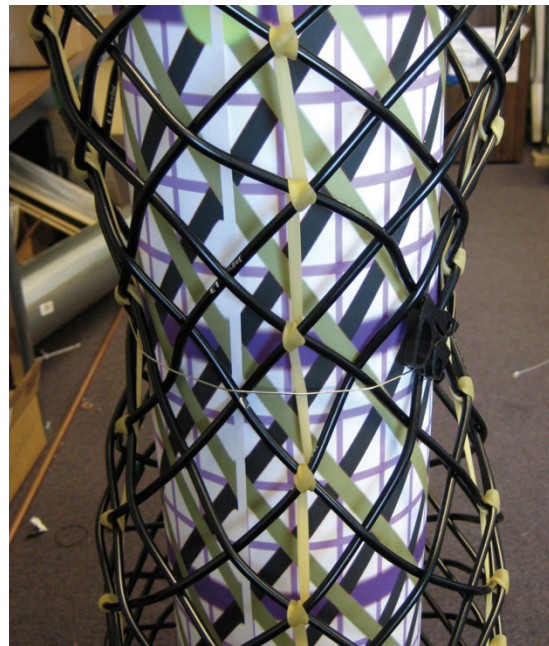
Figure 9: A hoop actuator created by a steel cable that runs through the brake cable sheathing.
