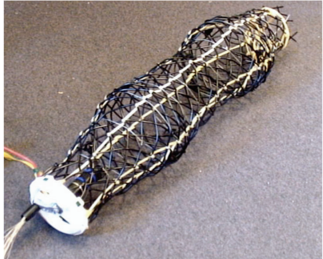
Figure 1: A video still from the first trial of a robot that creates peristaltic motion with a continuously deformable exterior surface.
