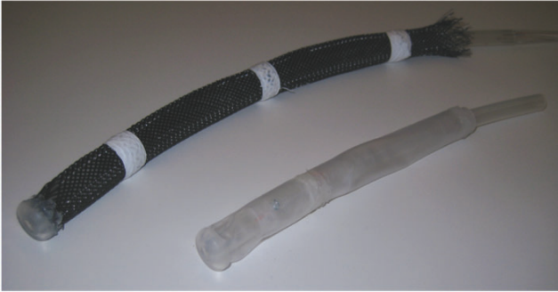
Figure 2: (Left) A previously built worm-like robot with discrete actuators surrounded by a braided mesh. (Right) The inner actuator core that inflates the mesh [6].
