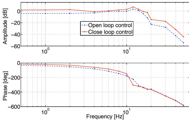
Fig. 5. Bode plot of the system in open and closed loop force control over a frequency range of 0.05 to 50  $Hz$ . The closed loop force control bandwidth is about 18  $Hz$ .
