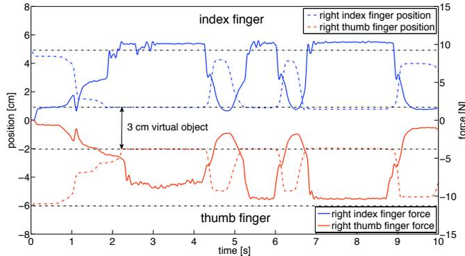
Fig. 6. Position (dashed) and force (plain) profiles for the index and thumb fingers during a pinch movement against a virtual object of 3  $cm$  width simulated by the *ReGrasp*.
