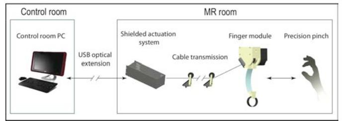
Fig. 7. Diagram representing the different components of *ReGrasp* combined with a shielded sensing and actuation box, from PC in the control room to the finger modules at the entry of the scanner bore, as it will be used in fMRI studies.
