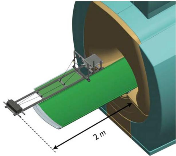
Fig. 3. Schematic of the *ReGrasp* placed within an MR room. The actuation system is placed about  $2\text{ m}$  away from the edge of the magnet, and contains all sensing and control hardware, eliminating the need for electronic components close to the magnet. Motor torques are transmitted to the finger modules over a cable transmission.
