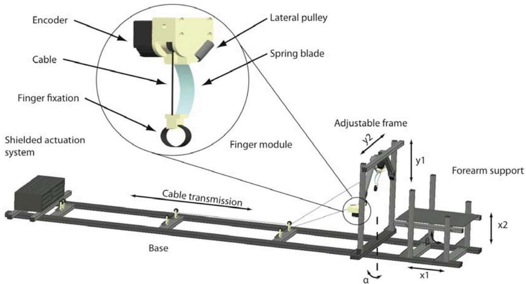
Fig. 2. The *ReGrasp* consists of two finger modules actuated over a stiff cable transmission, an adjustable frame to which the finger modules are fixed and an adjustable forearm support. Actuated over a remote unit containing a shielded conventional electromagnetic actuator [6], it can become a powerful neuroscience tool in conjunction with fMRI.
