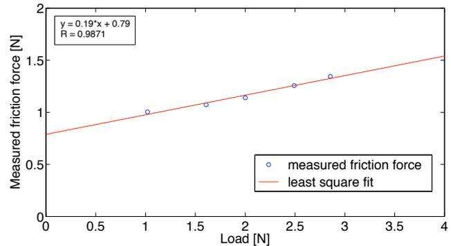
Fig. 4. Friction force in the cable transmission is measured for different loads applied at the finger fixation. Friction force is proportional to the load showing that mainly dry friction occurs in this system.
