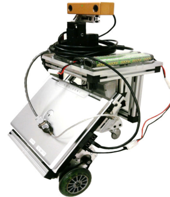
Fig. 1. Our experiments used an Evolution Robotics ER-1 (a two-wheeled differential drive robot) equipped with a pan-tilt unit and a stereo camera.
