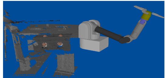
Fig. 5. A screenshot of the simulator illustrating the meshes used and typical results from the laser scanner.
