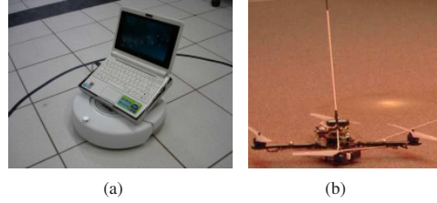
Fig. 4. Pictures of the robots: iRobot's Create (Fig. 4(a)) and quadrotor robot (Fig. 4(b)).
