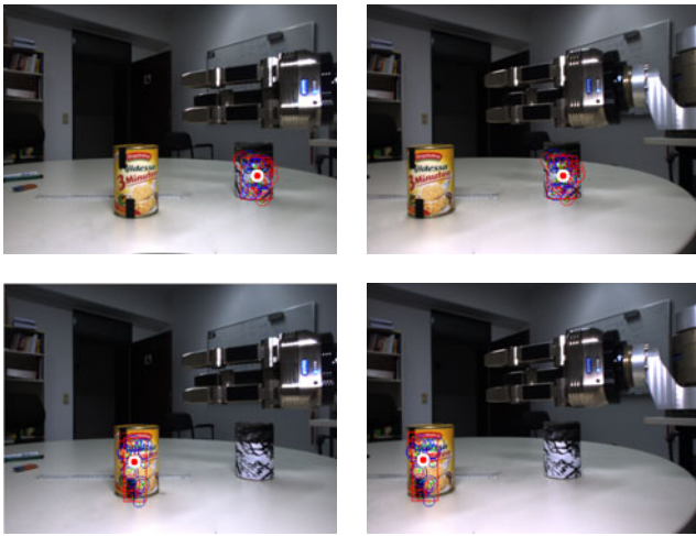
Fig. 2. Identifying and locating objects using SURF interest points and a stereo camera. Each row depicts the recognition of an object. The left and right column correspond to the left and right camera, respectively.
