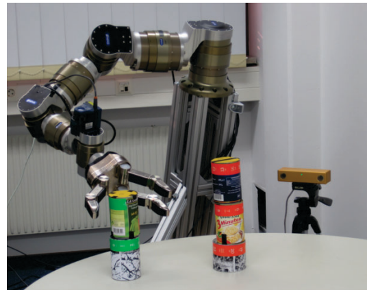
Fig. 1. The robot has successfully put objects with green and red labels into separate piles, using probabilistic inference on different levels of abstraction for planning and control.
