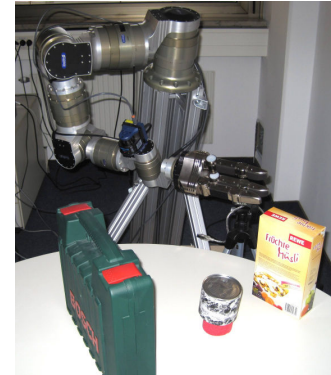
Fig. 1. The Schunk arm with the Hokuyo laser sensor mounted, in a scenario with a table and 3 other block obstacles. The goal is to reach the target, a point behind the cylinder in the middle.
