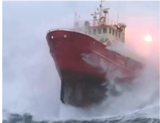
Fig. 1. A ship in high sea. The wave forces can result in very high accelerations in the ship motion.
