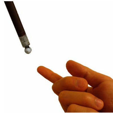
Fig. 1. Miniaturized triaxial optical fiber force sensor prototype.
