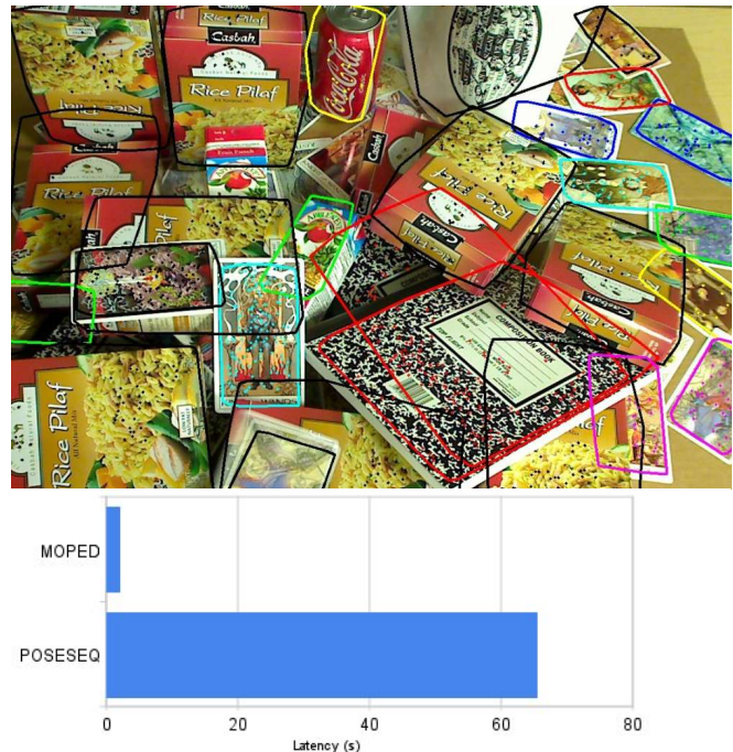
Fig. 1. A cluttered real-world scene. MOPED finds 27 objects partially-occluded, repeated and non-planar objects. The database contains 91 models and the source image is 1600x1200. In this scene, MOPED is 30.78 times faster than POSESEQ [3]
