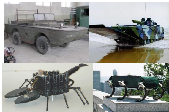
Fig. 2. Types of amphibian solutions. amphibian vehicles with wheel and track (top); Lobster Robot[2] and RHex/AQUA robot[3] (bottom)
