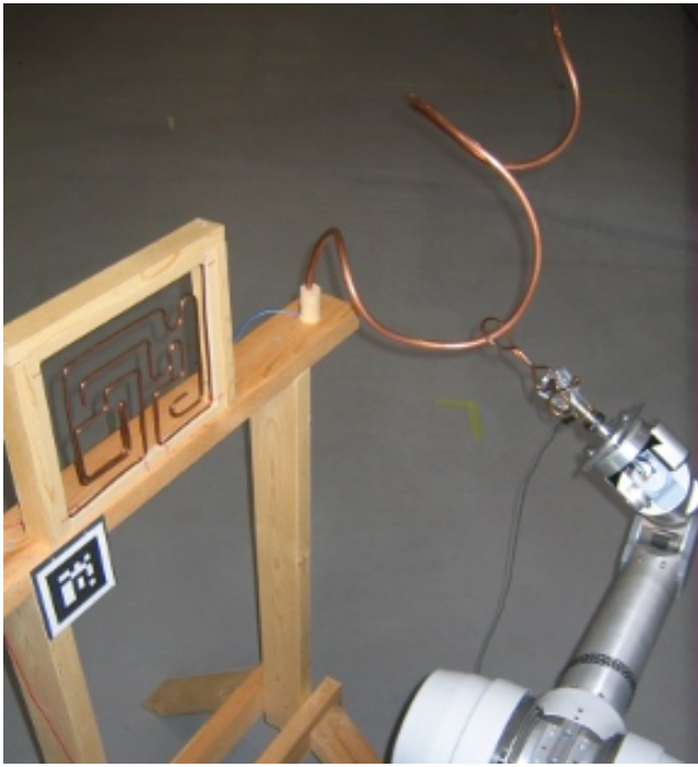
Fig. 6. The WAM manipulator, the wire maze (left) and the tube maze (right). The 2-D barcode in the lower-left is a visual fiducial used to detect the location of the rig relative to the robot. The rig and mazes are not modelled by the learning algorithm.
