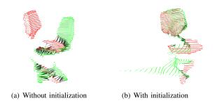
Fig. 2. Correspondences between two point clouds without the spin image initalization 2(a) and with the initialization 2(b). Without the initialization, ICP performs poorly when the two point clouds have a high rotational transformation as shown in 2(a). 2(b) shows that the same two sets match well with the initialization.
