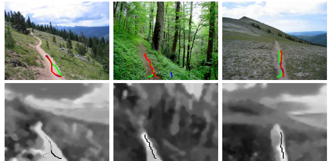
Fig. 1. Input images (above) and respective saliency maps (below), where saliency is represented in grey level. These maps are the superposition of two conspicuity maps, one for colour and the other for intensity channels. Each of these maps is searched for trails by agents (see Section II-B), whose paths are described by the overlaid lines. Thicker lines refer to the most probable trail candidate, which appears in the input image in red. The other coloured lines are from the best agent found on each conspicuity map.
