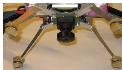
Fig. 2. The \mu Eye camera with a 190^\circ lens recording monochrome pictures from the surrounding of the helicopter. It is pointing downwards onto the ground.
