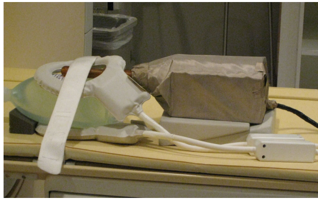
Fig. 5. Experimental setup for compatibility test in 3T MR scanner. Left image shows unshielded robot, phantom, and imaging coils. Right image shows shielded robot, phantom, and imaging coils.
