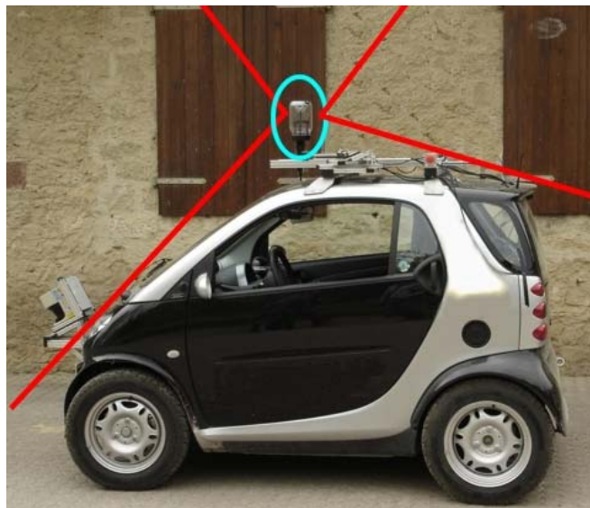
Fig. 5. The vehicle used in our experiments equipped with the omnidirectional camera (in the circle). The vertical field of view is indicated by the lines.
