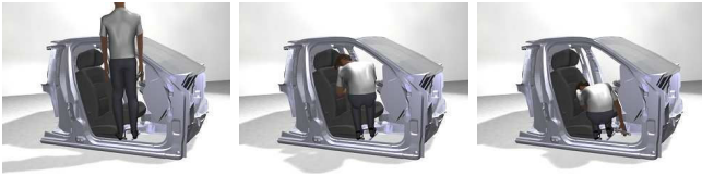
Fig. 8. Bending: 41-DOF human-shape robot bends and stretches to put the tool inside the car. Retraction algorithm’s maximum speedup is 2 times and can succeed when non-retraction planner fails.
