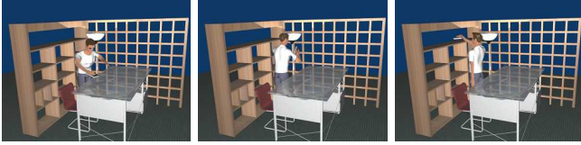
Fig. 7. Placing Object: 41-DOF human-shape robot picks the book and puts it on the shelf. Retraction algorithm’s maximum speedup is 4 times and can succeed when non-retraction planner fails.
