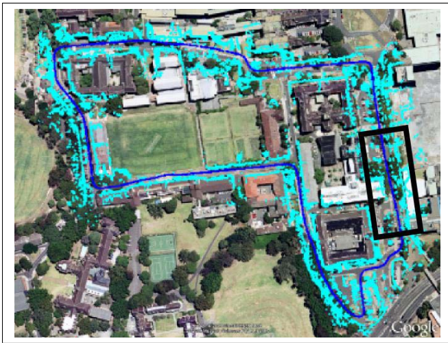
Fig. 7. Satellite view of scanned region with laser returns indicated
