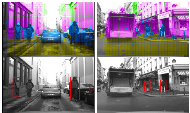
Fig. 10. Structure and Appearance Classification. The first row shows the result of structure classification; the second row shows the final classified boxes.
