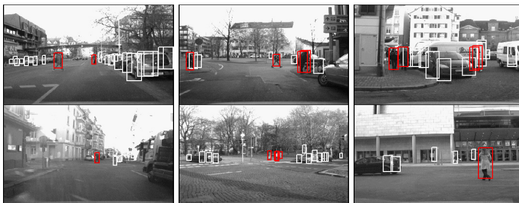
Fig. 11. Examples of pedestrian classification showing coverage at different distances upto 40 m. White boxes denote the output of the stereo-based pedestrian detector after structure classification. Red boxes denote the final pedestrian classifications. The last image shows an example of a failure of our system for the furthest pedestrian.
