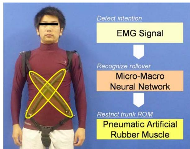
Fig. 1. Intelligent trunk orthosis to support rollover. Note that, in this orthosis, the rollover is recognized using the EMG signal and the original neural network. After that, rollover is supported by restricting trunk rotational movement using the pneumatic artificial rubber muscle
