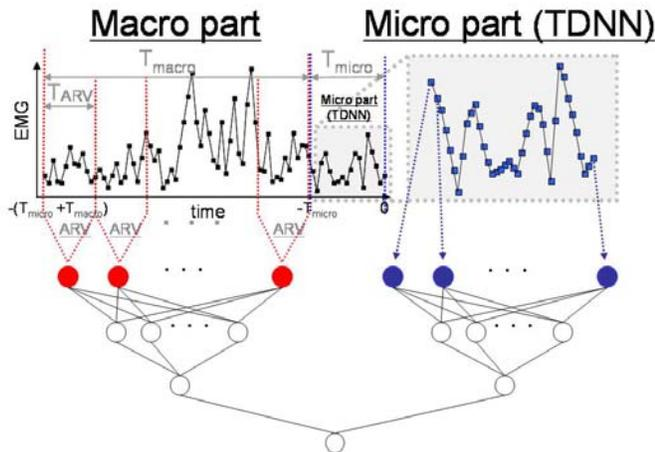
Fig. 2. Micro Macro neural network. Note that MMNN is divided into the Micro Part and the Macro Part.
