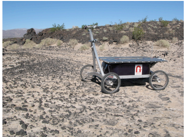
Fig. 1. Robotic explorer, Zoë, in the Amboy Crater lava field. Stereo cameras enable obstacle detection and terrain modeling for navigation. Additional high-resolution cameras and visible/near-infrared spectrometer collect measurements of rocks and soil for classification and geologic mapping.
