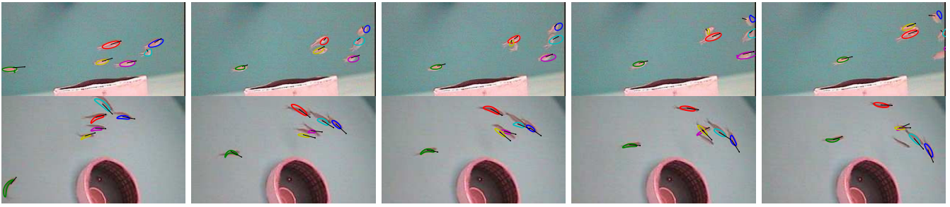
Fig. 6. Tracking results for shape. The bent ellipsoid shape is projected back onto two cameras at five different time-steps. Black arrows represent heading. A target track is lost during occlusion in the 30th frame
