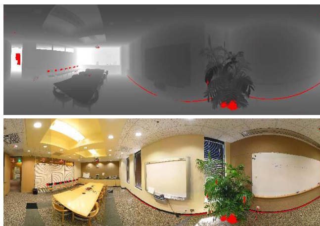
Fig. 3. Panoramic range image (top) and texture image (bottom) with 1/2 degree resolution. Invalid cells are marked red.
