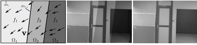
Fig. 8. The texture blending globally optimizes the texture color and removes discontinuities at boundaries between texture regions reconstructed from different camera images. The image in the middle shows the reconstructed texture and the right image the texture after blending.
