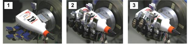
Fig. 5. Enfolding an object: (1) The object is laid into the opened robot hand. (2) The proximal phalanges of the robot hand are closed. (3) Finally, the distal phalanges are closed as well.
